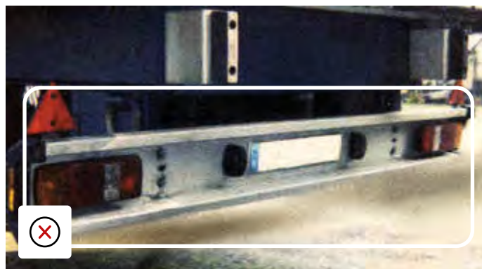
Under run guard bent & requires repair
