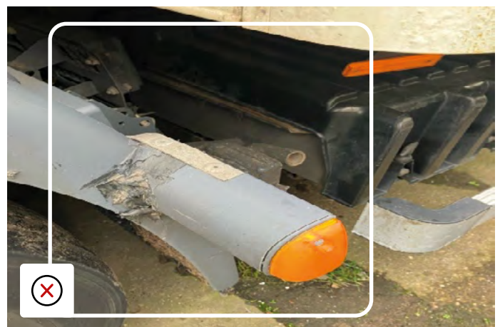
Substandard repair to side repeater mounting
