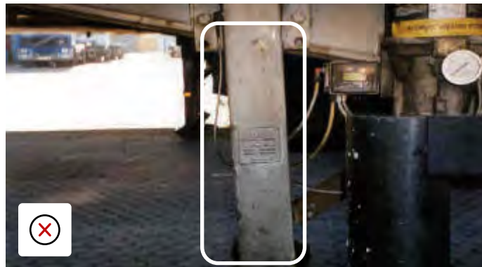
Landing leg bent & needs to be replaced
