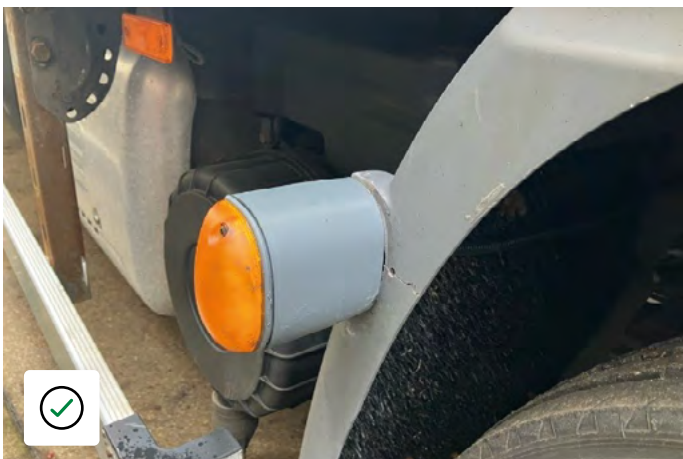
Side repeater & mounting in acceptable condition
