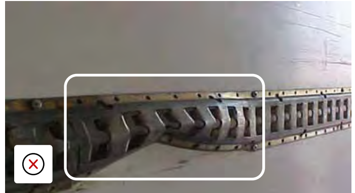
Interior load control damaged beyond repair.
