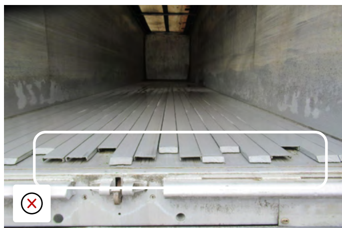
Bar edges are missing - goods can fall under the floor
