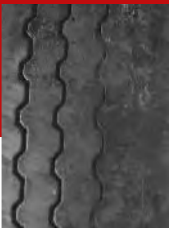
Uneven wear due to misalignment or camber
