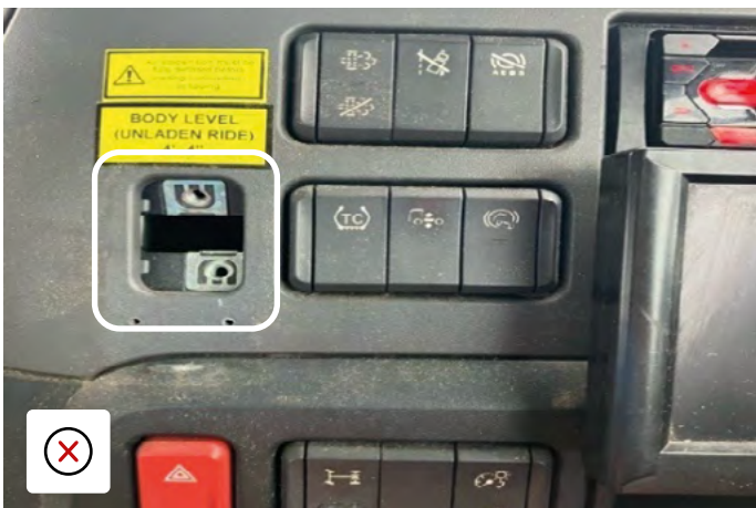
Screw holes in dash & trim missing
