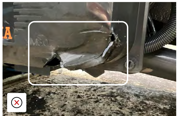
Cover broken - requires replacement
