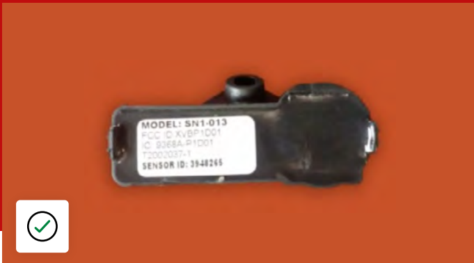
TPMS sensor in an acceptable condition
