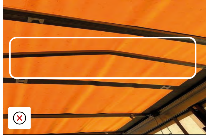
Edscha roof bows bent due to weight imposed from above.
