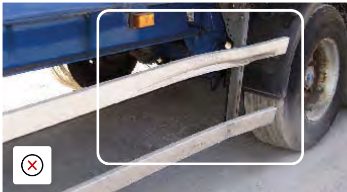
Impact dents and distortion to Aluminium side guard.
