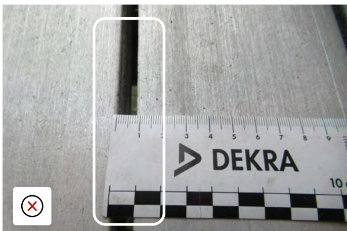
Floor bars spread and not safe for transport - goods can fall through the floor
