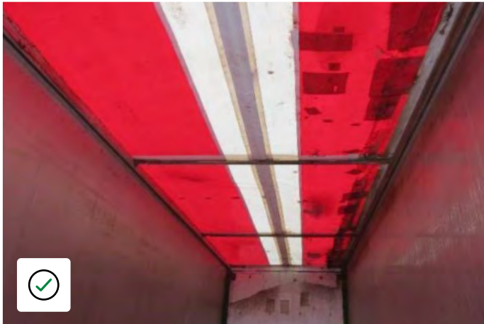
Roof sheet with minor patches to acceptable standard
