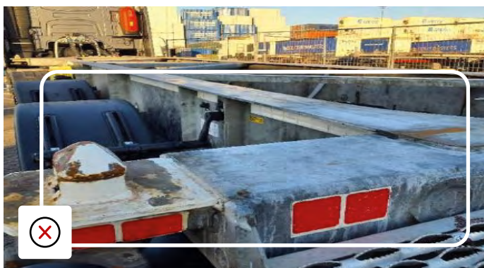
Chassis with containment requiring specialist cleaning
