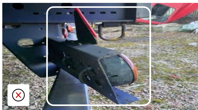
Lamp arm bent & requires repair
