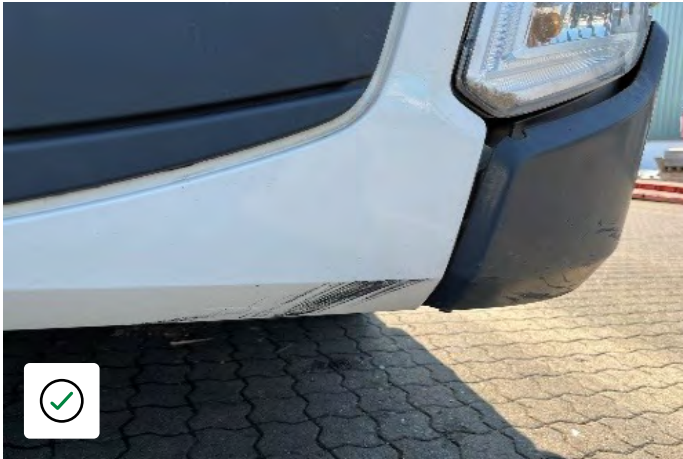
Minor scrape - no damage to the structure
