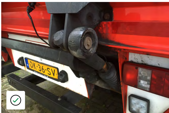
Platform roller with minor wear and tear
