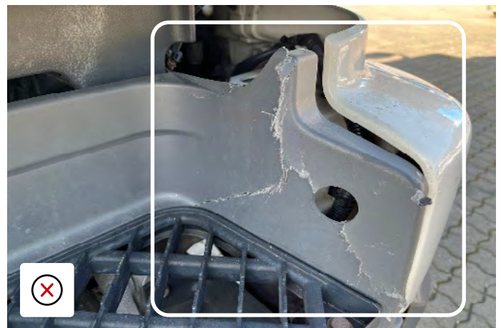
Step support structure unsafe due to impact
