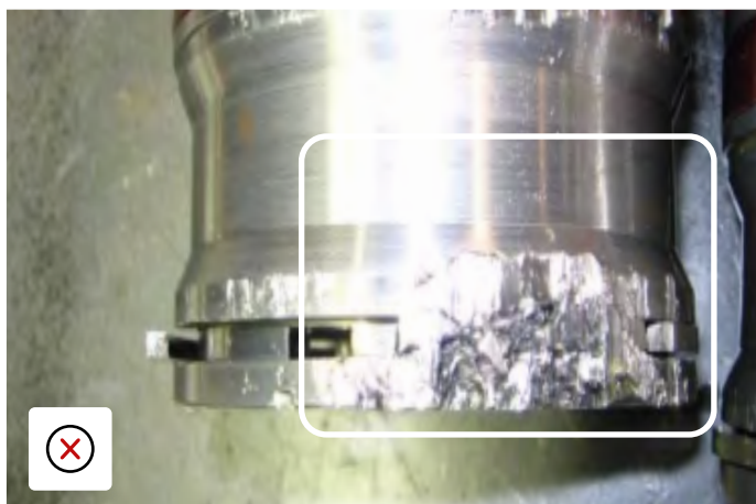
Hydraulic fittings with damage due to misuse & impact
