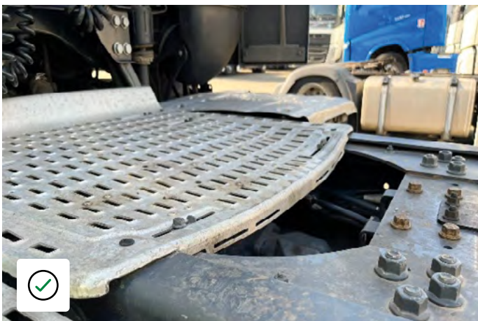
Minor deformation through normal wear & tear
