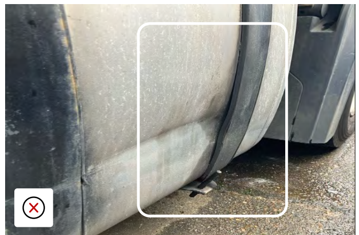
Fuel tank has been impacted & left large scrape
