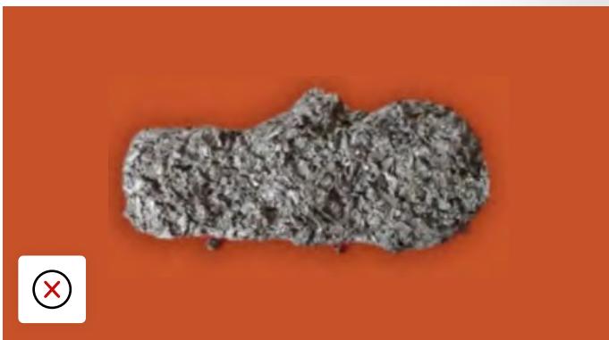
TPMS sensor contaminated by sealant
