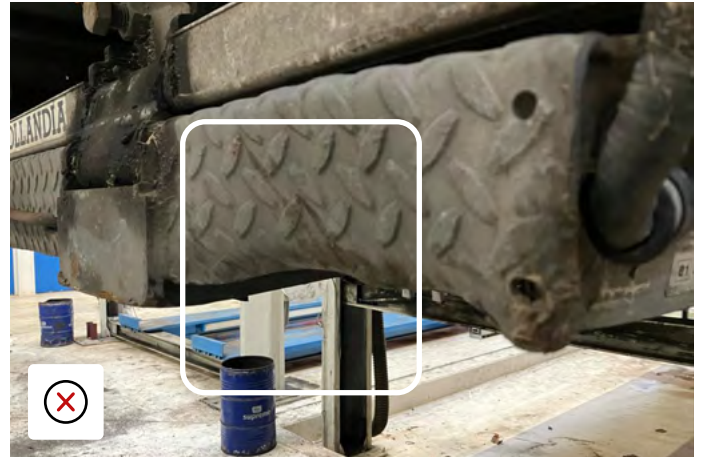
Platform impacted at a critical section - requires repair
