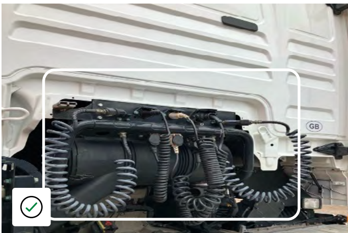
Suzie couplings in good condition & correctly stored
