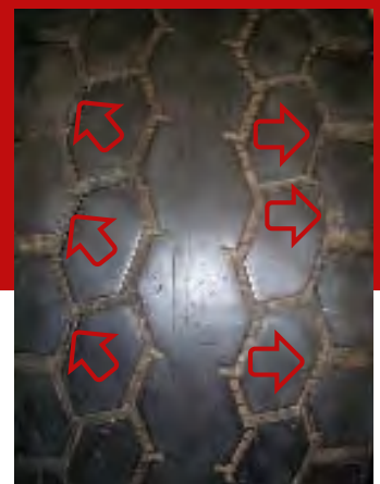
Tread groove cracking due to over inflation
