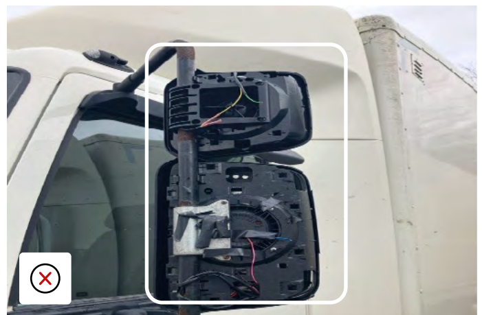
Mirror backing completely missing
