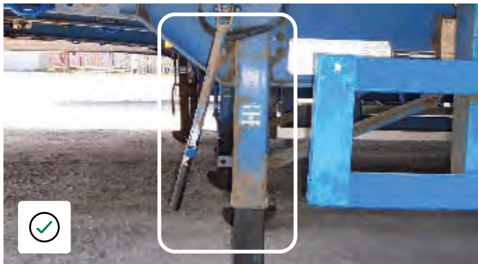
Landing leg straight with handle secure.
